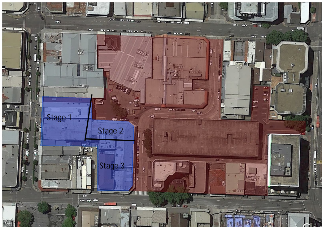
Figure 7-6: Proposed staging of the demolition works
