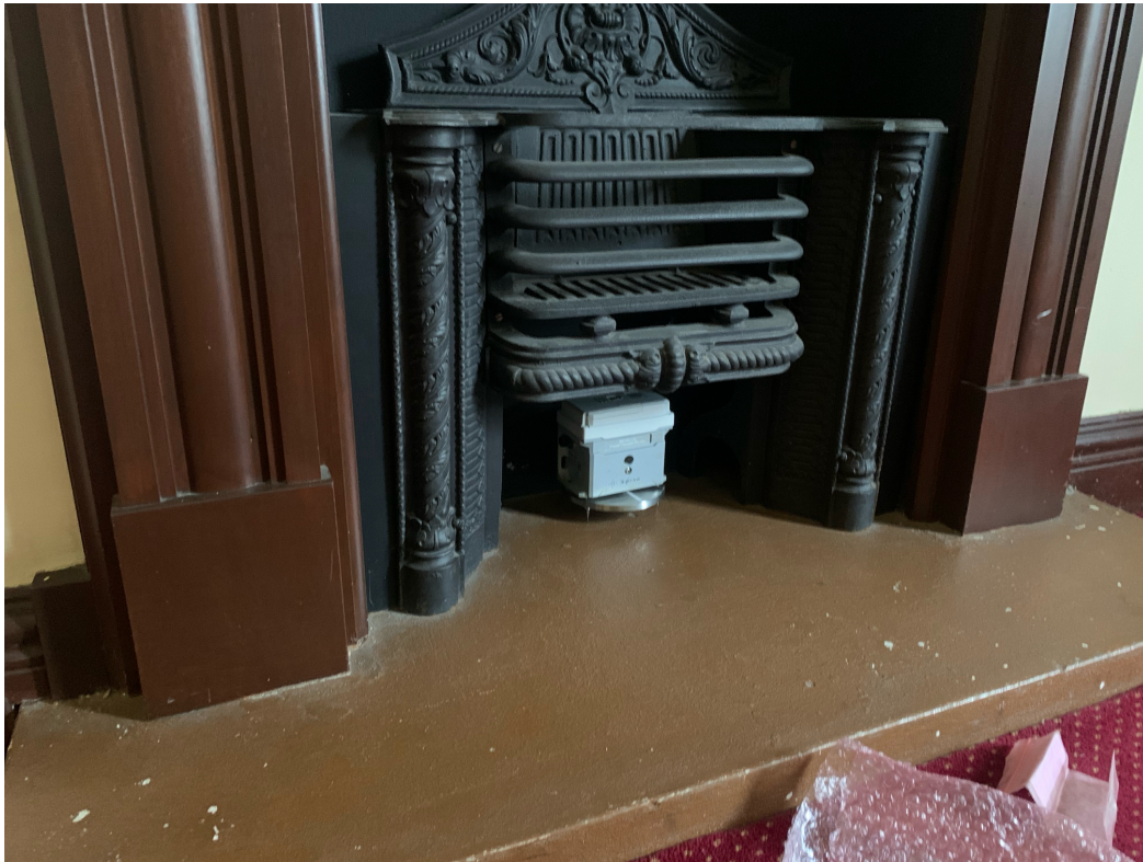
Figure 3: C22 Vibration Monitor (Kia Ora)
